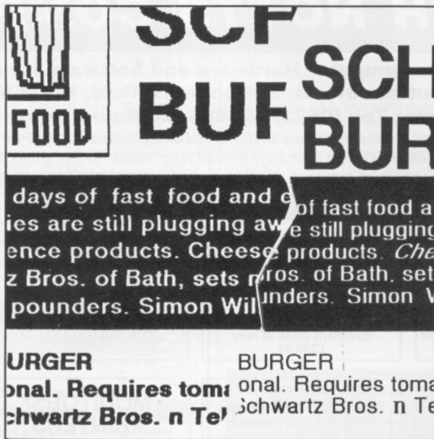
■ A close up of some output from Timeworks. The left side is on an Epson LQ850 24-pin dot matrix printer, the right side on the Atari SLM804 laser printer for comparison. You can see the higher quality of the laser, although PostScript output is better still.
